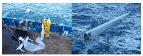
Fig. 3. A high-speed Manta trawl. (© Crown copyright 2011, permission granted by Cefas)
