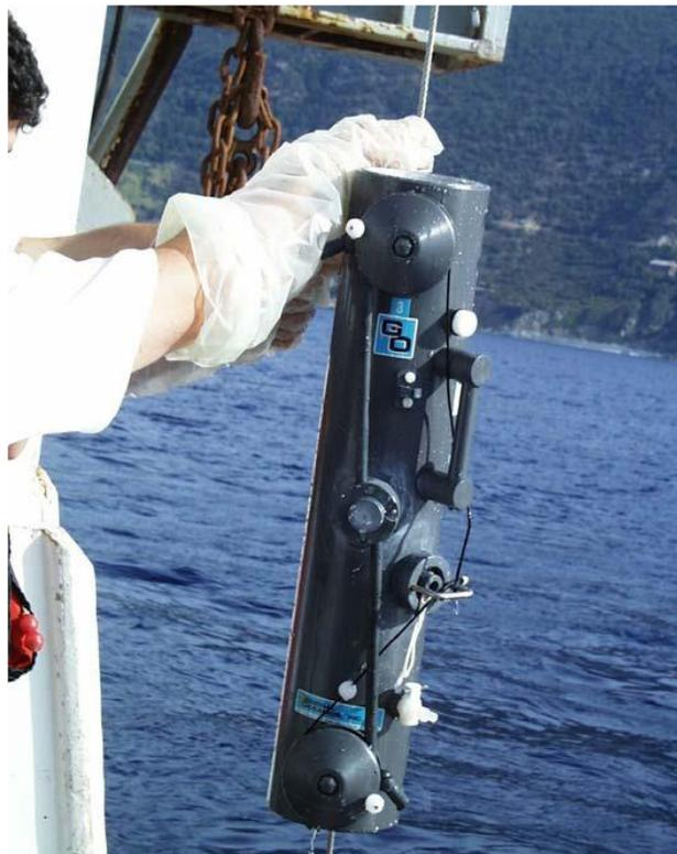
**Figure 1** Picture of a GO-FLO sampler (photo courtesy of IFREMER, France).
